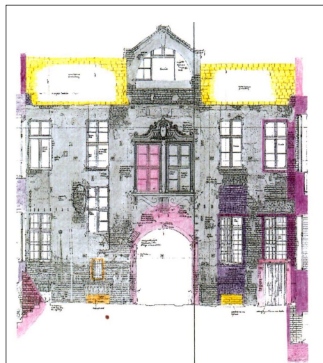
Picture 3.18: The house 11 Gipsstraße: With grey we can observe the parts of the house that are from 1800. The changes are marked with colour.
