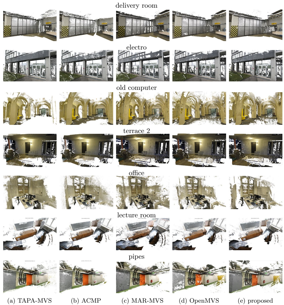
Figure 6.13: Qualitative point cloud comparison of our method with the state of the art baselines for the ETH3D training and test sets. Dense models for the state of the art methods are as in ETH3D evaluation site.
