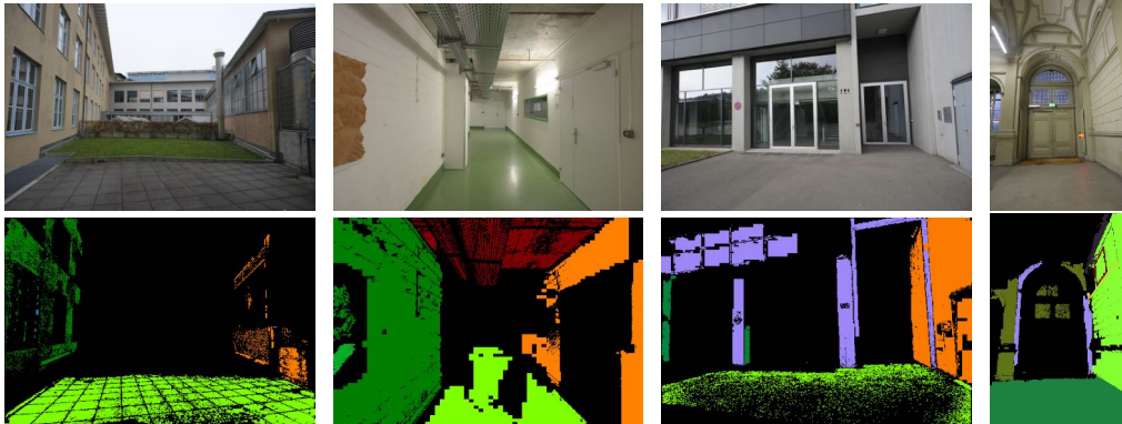
Figure 6.7: Generated plane prior hypotheses. Example images from ETH3D dataset (up) and the corresponding 3D plane hypothesis detected using the proposed RANSAC-based approach (bottom). Prior planes are color-coded by normal vector. Black regions refer to pixels with no assigned prior hypothesis.
