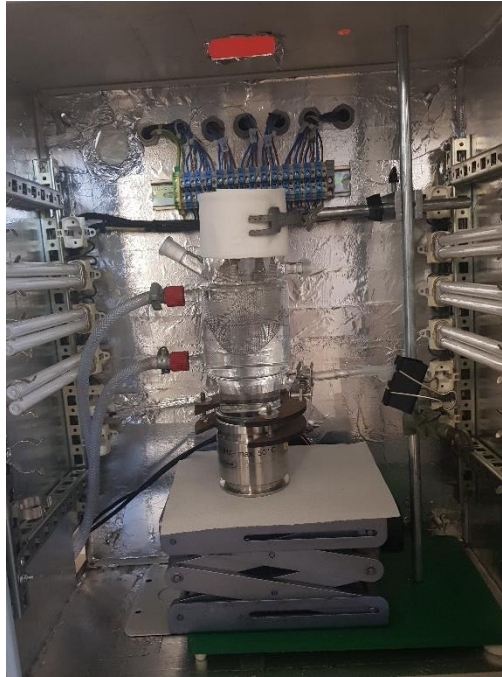
Figure 19. Combination of UV treatment and high frequency sonication – experimental setup.
