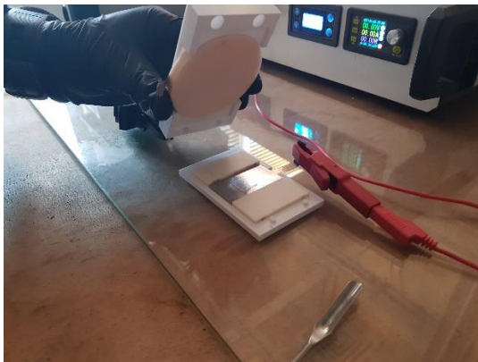
Figure 20: DBD plasma reactor – sample placement.
