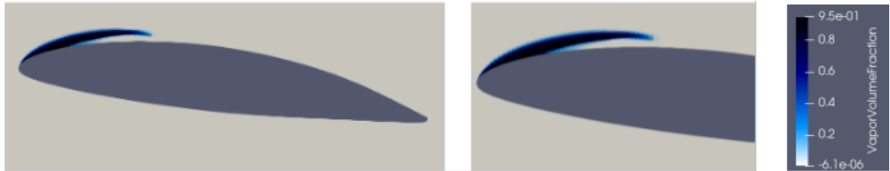
Figure 4.25: Vapor Volume Fraction around NACA66MOD for \sigma = 0.91
