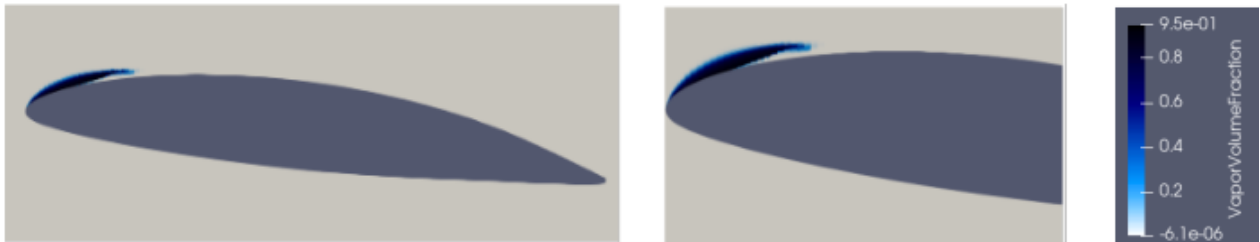
Figure 4.24: Vapor Volume Fraction around NACA66MOD for \sigma = 1
