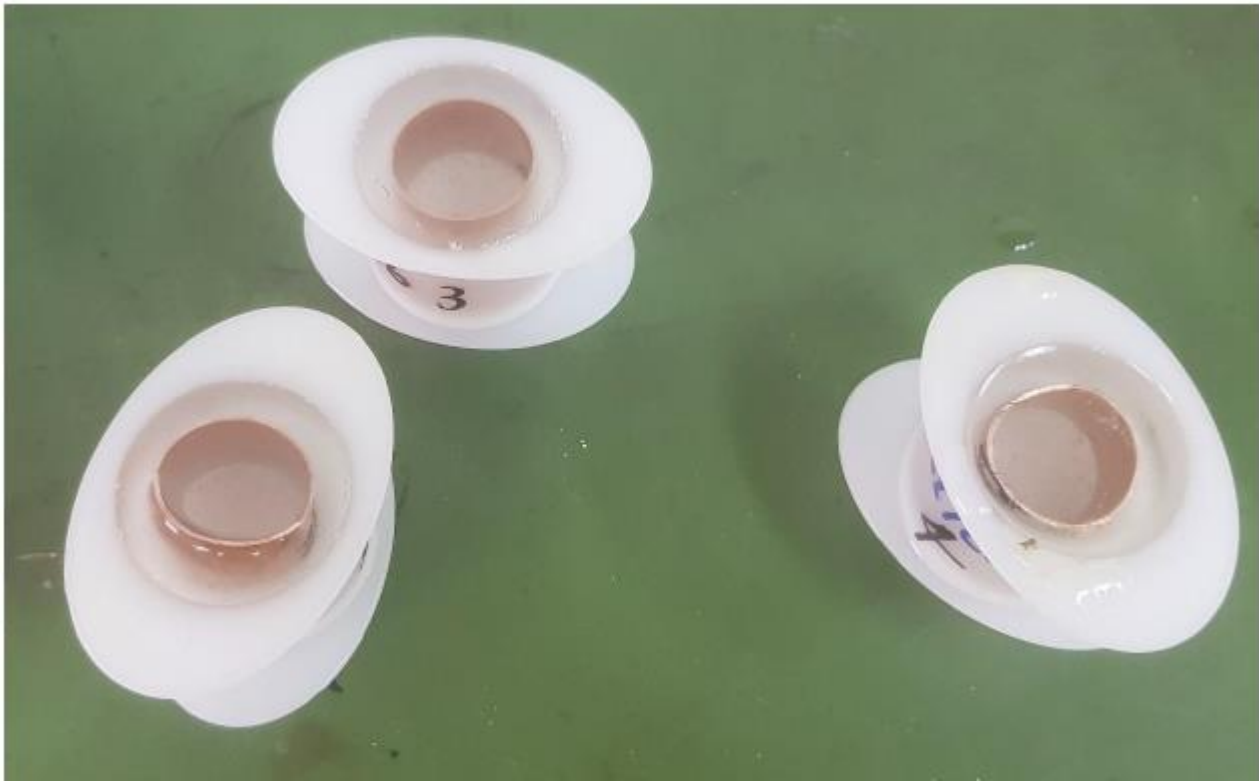
Image 33: Mounting specimens be prepared to metallographic examination
