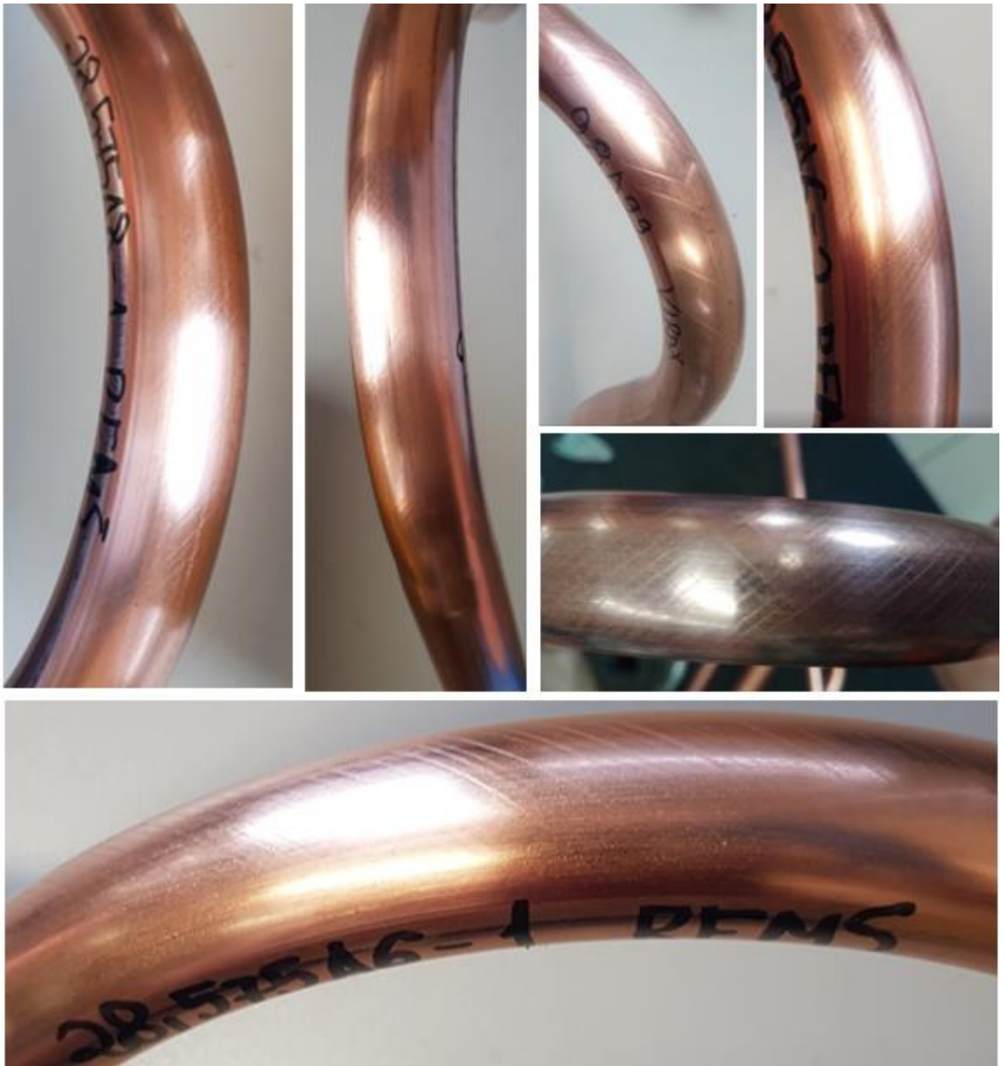
Image 13: Detailed Lueders Lines photos (Front & Top View)
