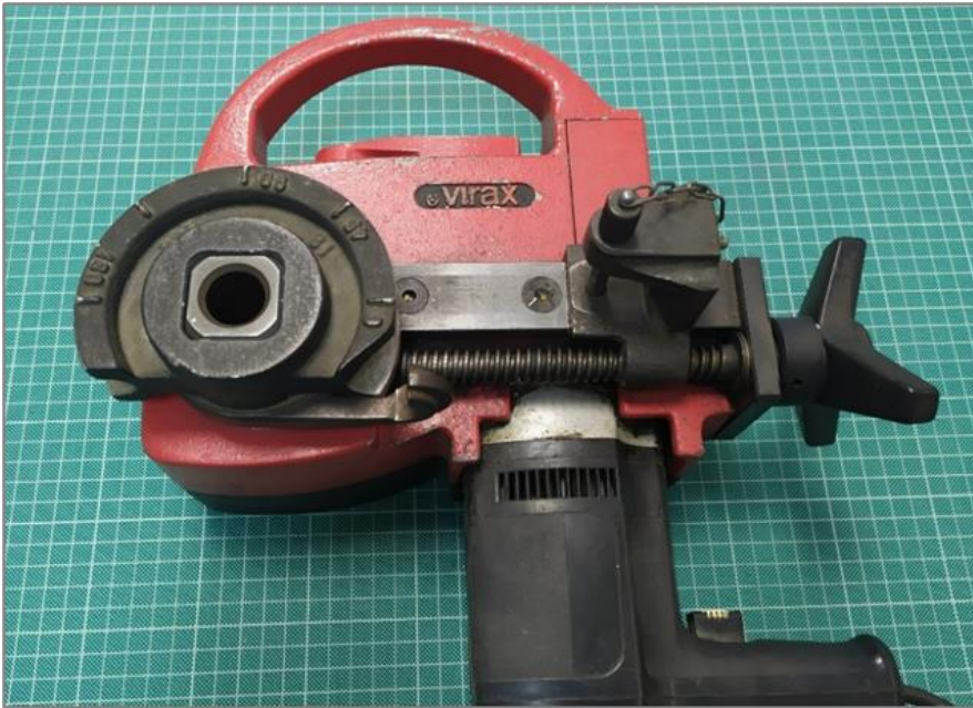
Image 7: Top view of Virax - Epernay bender
