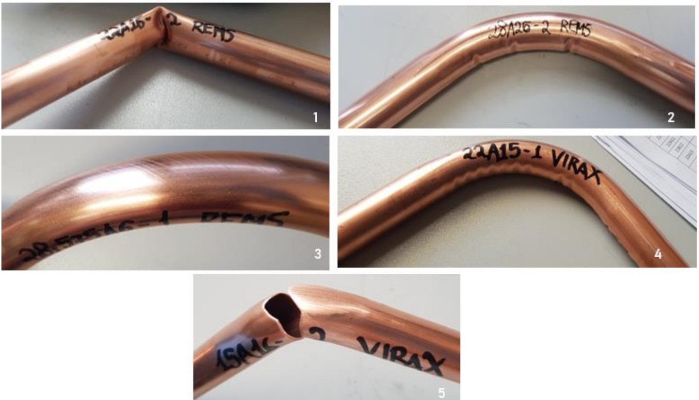
Image 12: Defects due to bending: (1) Buckling, (2) Kinking, (3) Lueders Lines, (4) Wrinkling, (5) Crack
