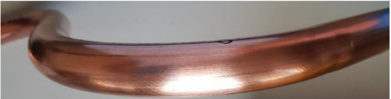
Image 44: 28,575A8 – 2 REMS hard copper tube's upper surface indicating Luder Lines
