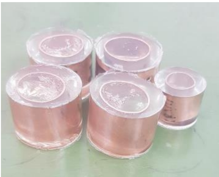
Image 34: Cured samples after the mounting procedure
