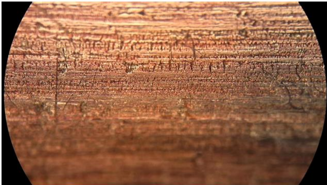
Image 48: Outer surface of a non – defected tube at the same point ( \times 100 )
