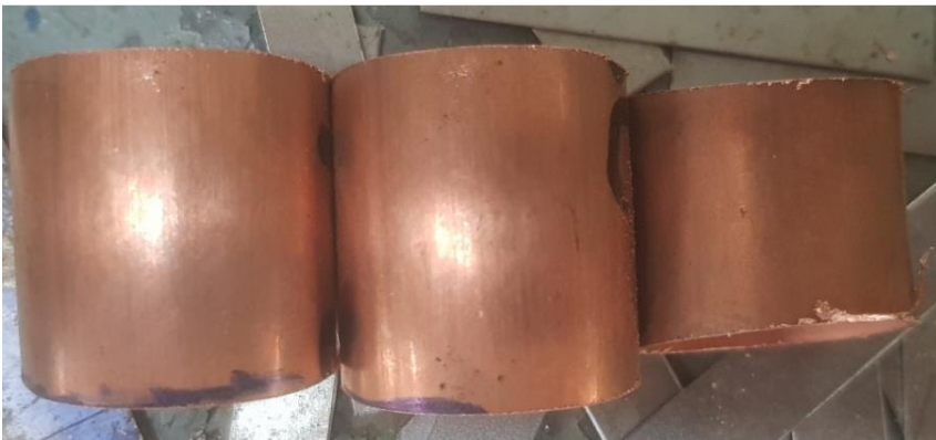
Image 16: Hard copper tubes' rings that have formatted slight Luder Lines
