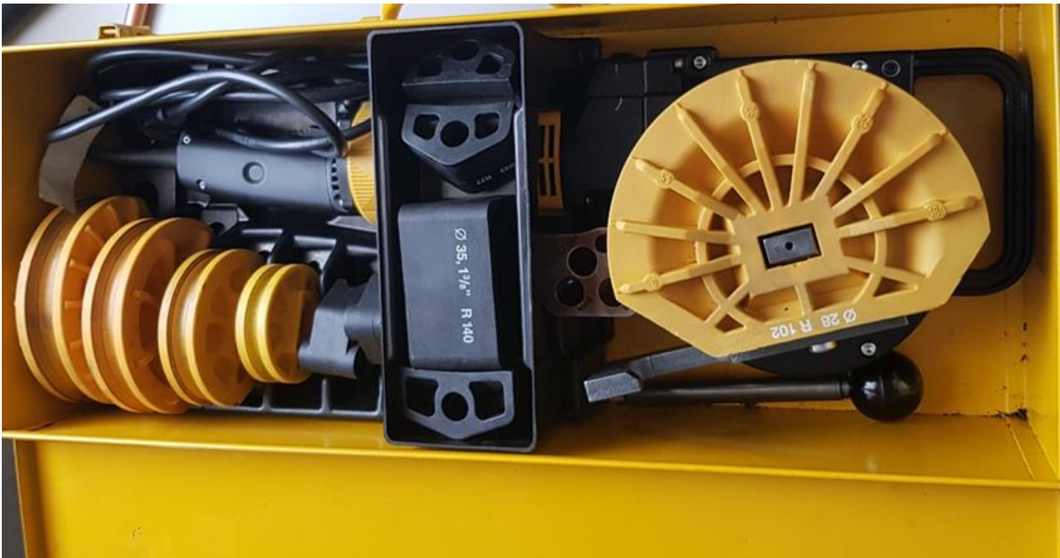
Image 9: REMS – CURVO removable dies according to the outer diameter of the tube
