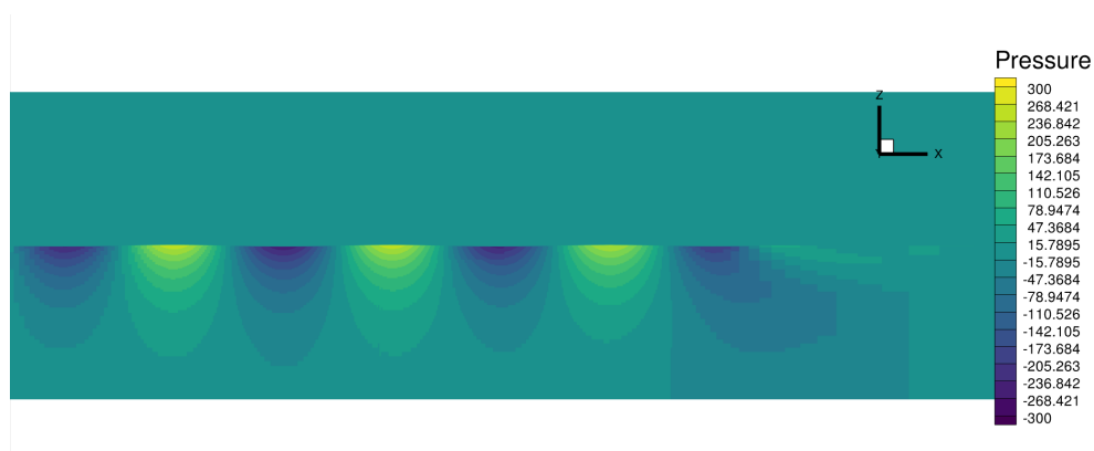
Figure 4.11: Contour Plot of the dynamic component of the pressure field in [Pa] .
