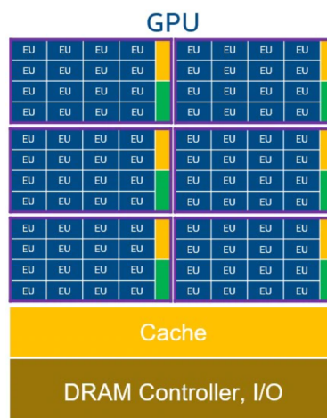
Figure 21. Each EU can process multiple SIMD instruction streams. Multiple EUs combine to form a compute unit with shared local memory and synchronization mechanisms [16].
