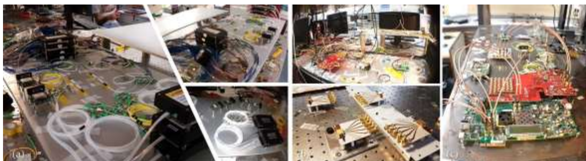
Figure 5: Photos of the demonstrator during the preparation period. (a) The POD switch, including a WSS with the “Demultiplex, switch and Multiplex” approach. (b) The fast tunable lasers used for the transmitter. (c) The FPGA boards that assemble the ToR switch
