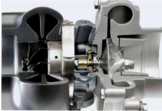
Figure 1.8: Full-floating ring fluid bearing-rotor system, taken from [63]
