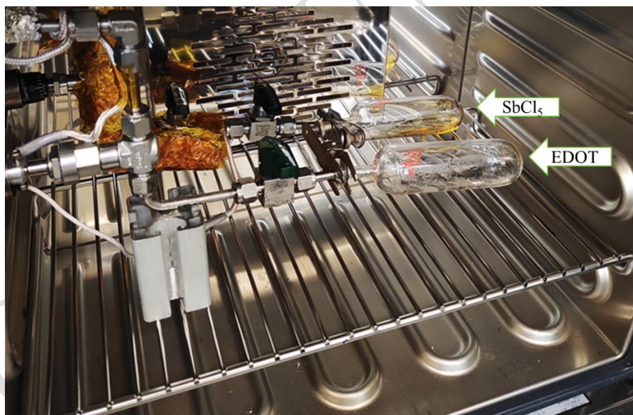
Figure 10: The \text{SbCl}_5 and EDOT reservoirs inside the oven.
