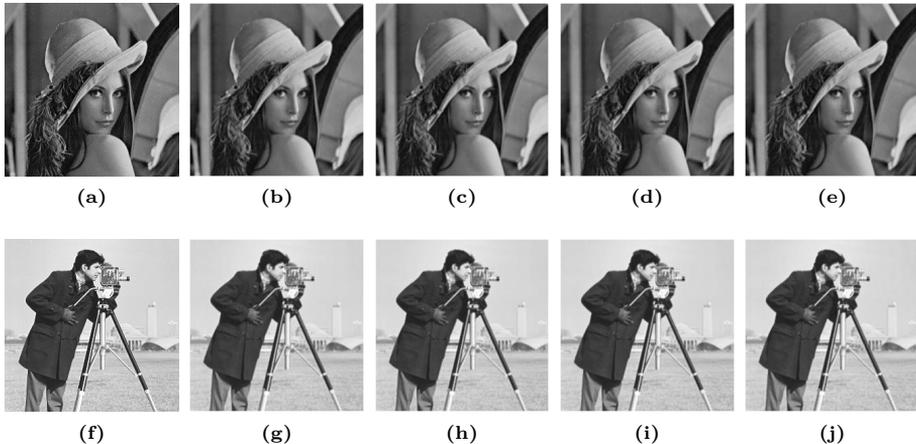
**Figure 7.8:** I/O images of approximate Gaussian blurring: (a),(f) input images, and output image with (b),(g) accurate multiplier, (c) AxFPU16<sub>|1,0</sub>, (d) AxFPU16<sub>|3,4</sub>, (e) AxFPU16<sub>|4,6</sub>, (h) AxFPU32<sub>|4,12</sub>, (i) AxFPU32<sub>|6,14</sub>, (j) AxFPU32<sub>|10,18</sub>.
