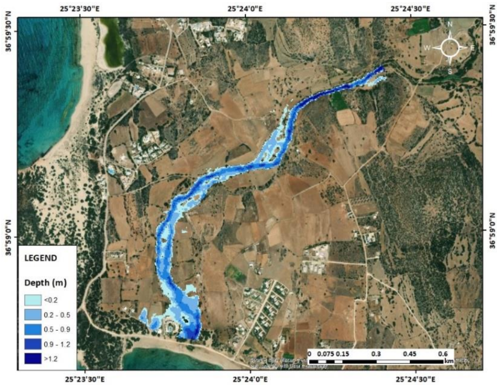
Figure 13: Maximum depth floodplain of 2 nd subbasin with Time-Area method
