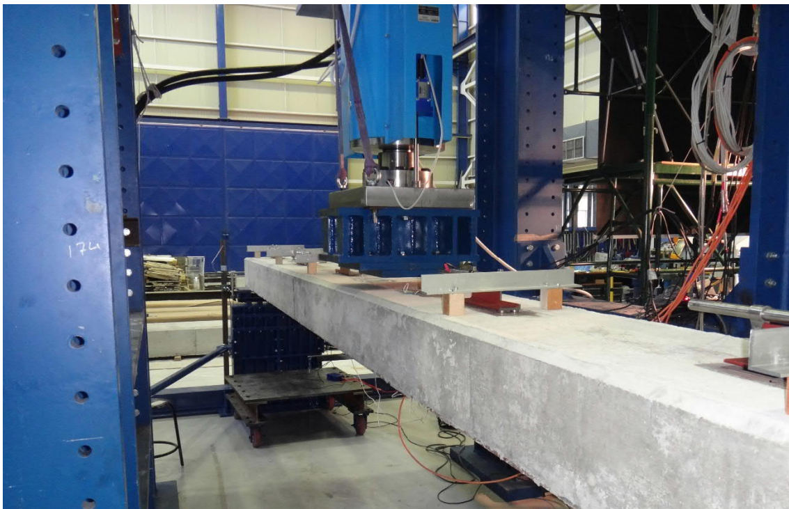
Fig. 4.31- Rigid block at the bottom of the loading actuator
