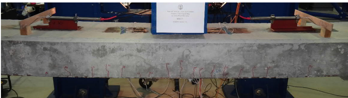
Fig. 5.51- S1- Cracks at deflection of 50 mm (fig. 5.57 and 5.58, points B and B')
