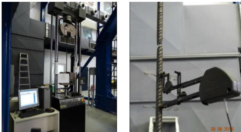
Fig. 4.16- Set-up for the tensile tests of the bars
