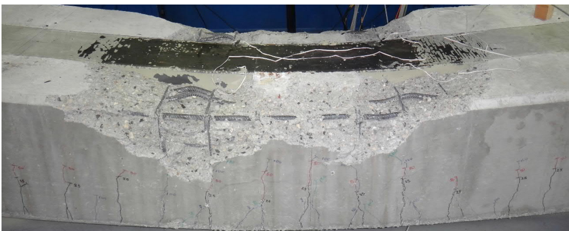
Fig. 5.70- S11- The specimen at the end of the test (fig. 5.71 and 5.72, points G and G')
