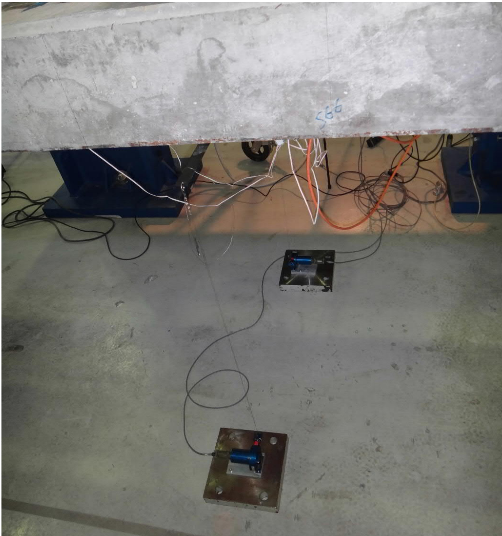
Fig. 4.32- Wires for the measurement of deflection at the mid-span
