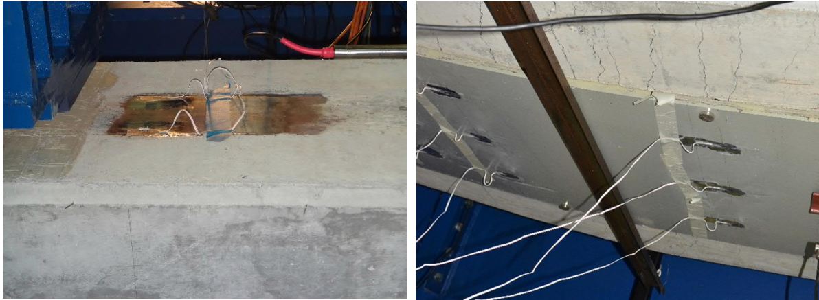
Fig. 4.35- Strain gauges at the top (left) and bottom (right) plates
