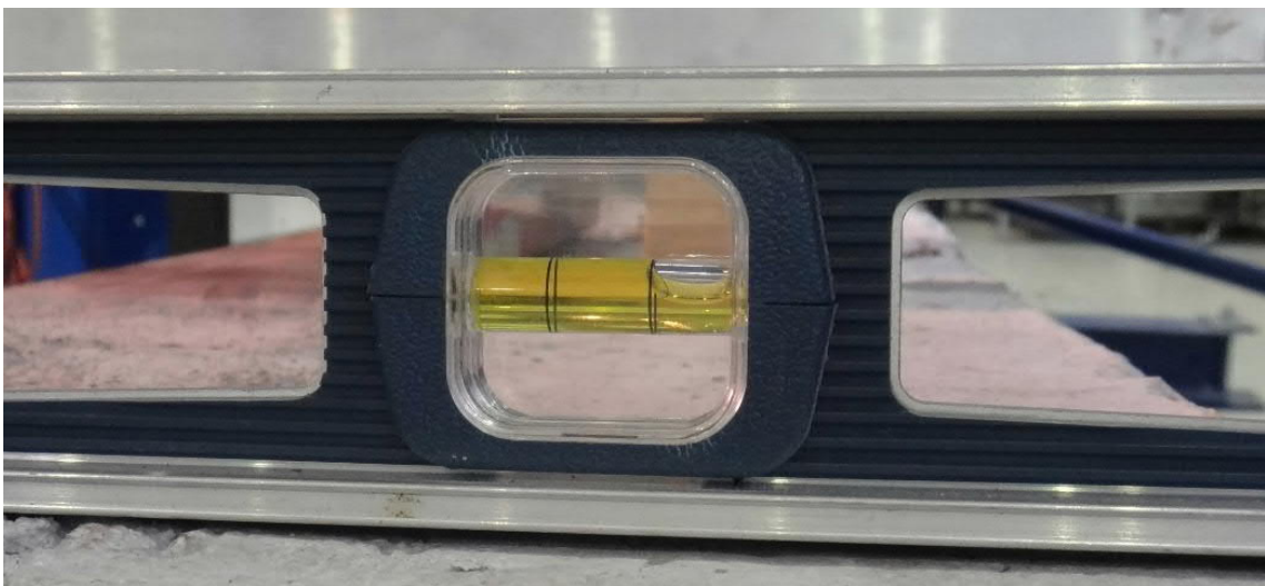
Fig. 5.83- S12- Torsion at the end of the test (fig. 5.85 and 5.86, points E and E')
