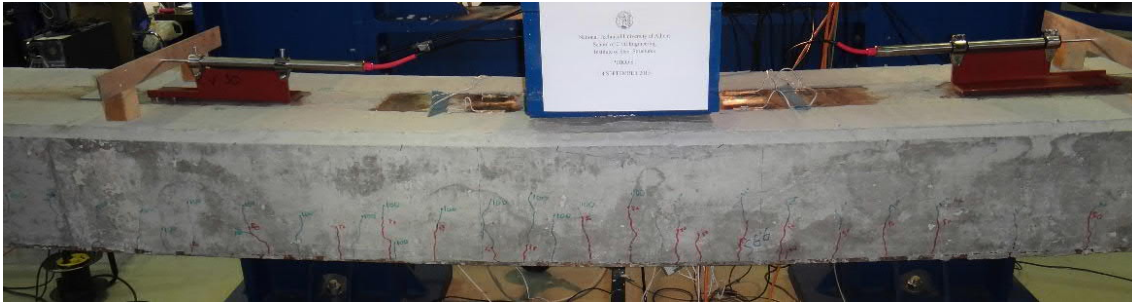
Fig. 5.52- S1- Cracks at deflection of 100 mm (fig. 5.57 and 5.58, points D and D')
