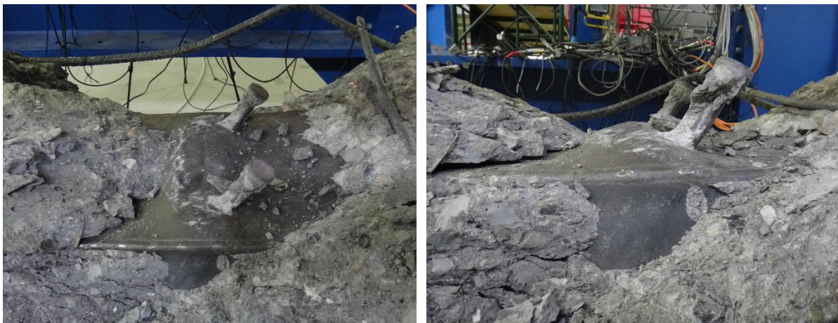
Fig. 5.41- S5- Buckling at the top plate of the steel beam
