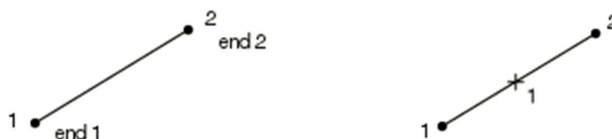
Fig. 6.8- Node ordering on elements (left) and integration point for output
