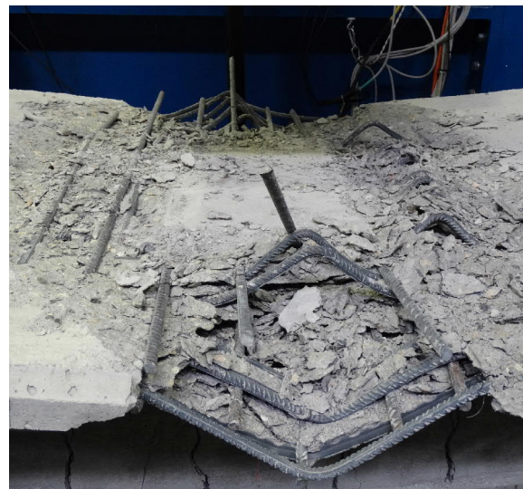
Fig. 6.59- S10- Deformed shape on FE model (left) and specimen at the end of the test (right)
