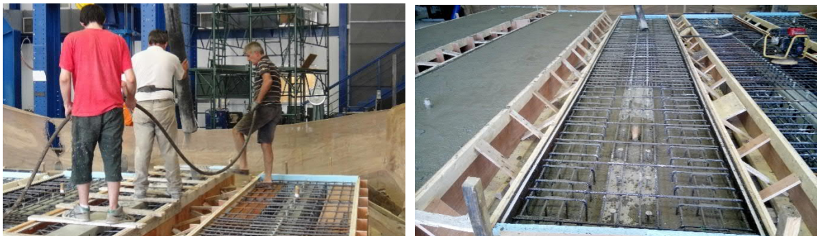
Fig. 4.14- Concreting of specimens
