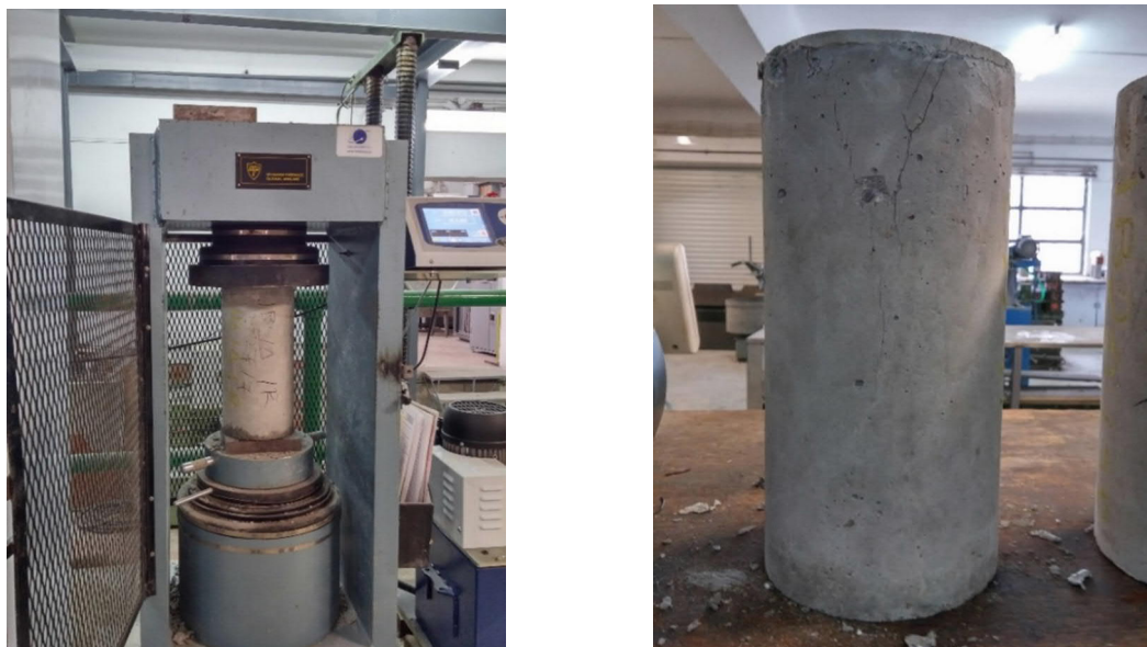
Fig. 4.20- Compression tests of the concrete specimens
