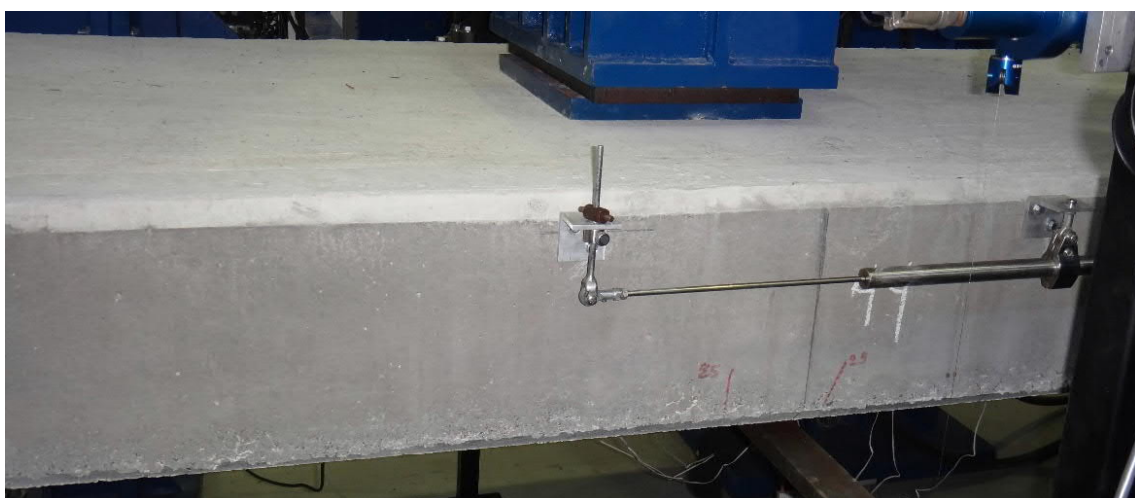
Fig. 5.94- S6a- Cracks at deflection of 25mm (fig. 5.104 and 5.105, points A and A')
