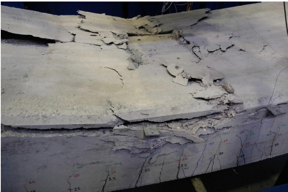
Fig. 5.141- S8- The beam at the end of the test (fig. 5.144 and 5.145, points G and G')
