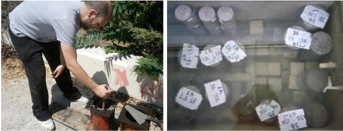
Fig. 4.18- Creating the cylindrical specimens
