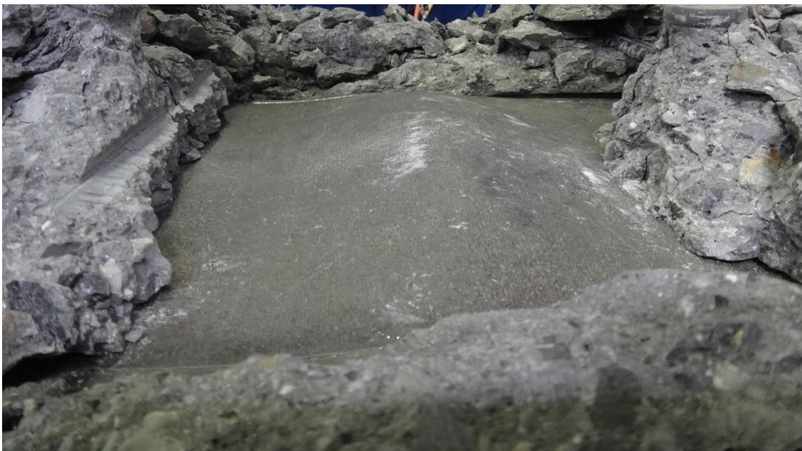
Fig. 5.29- S4- Buckling at the top plate of the steel beam
