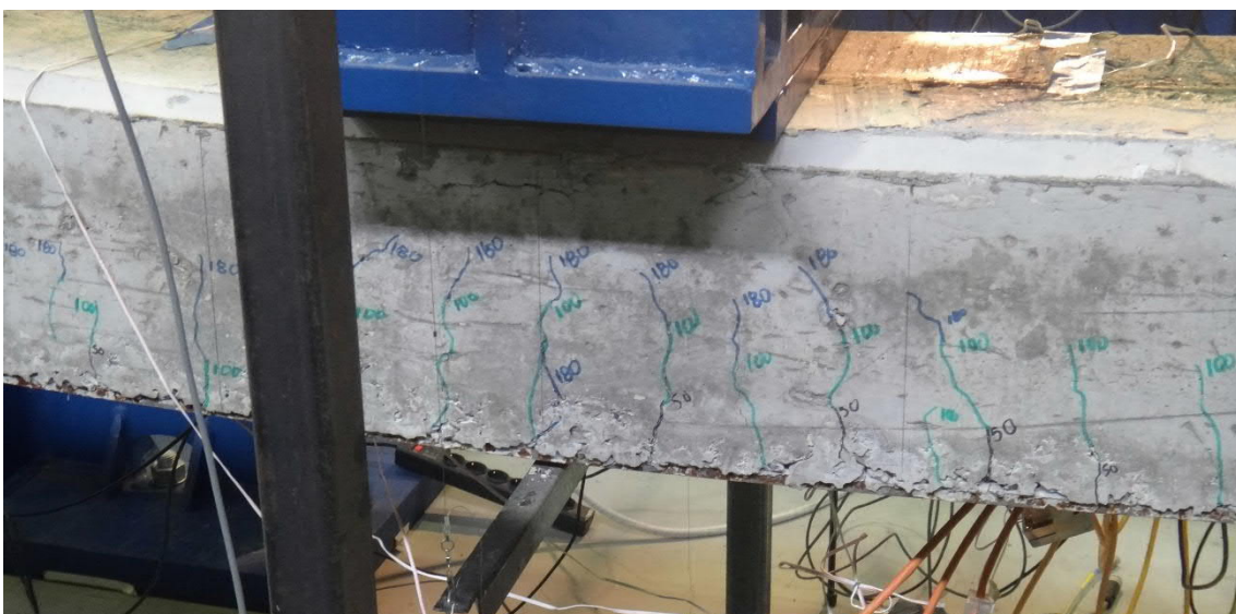
Fig. 5.81- S12- Cracks at deflection of 180 mm (fig. 5.85 and 5.86, points D and D')
