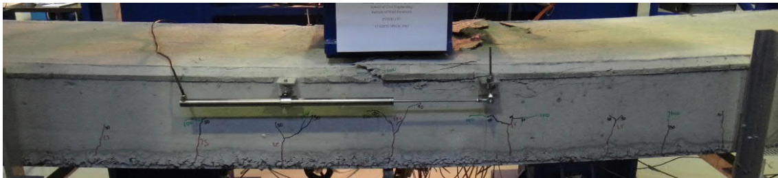
Fig. 5.3- S2- Tensile and compressive cracks at deflection of 117 mm (fig. 5.6 and 5.7, points C and C')
