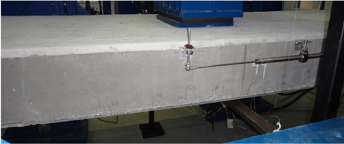
Fig. 5.95- S6a- Cracks at deflection of 50mm (fig. 5.104 and 5.105, points B and B')
