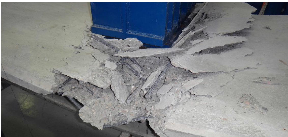
Fig. 5.169- S10- The beam at the end of the test (fig. 5.172 and 5.173, points E and E')
