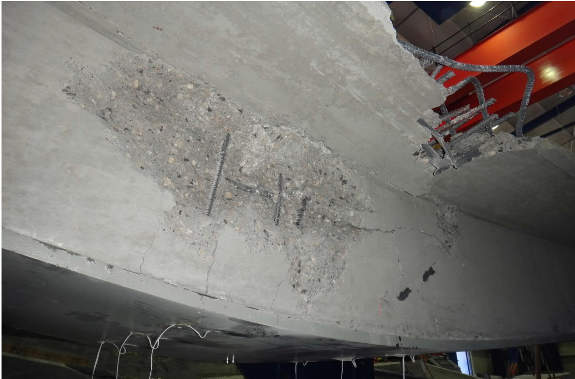
Fig. 5.170- S10- Cracks at the middle of the span at the end of the test (fig. 5.172 and 5.173, points E and E')
