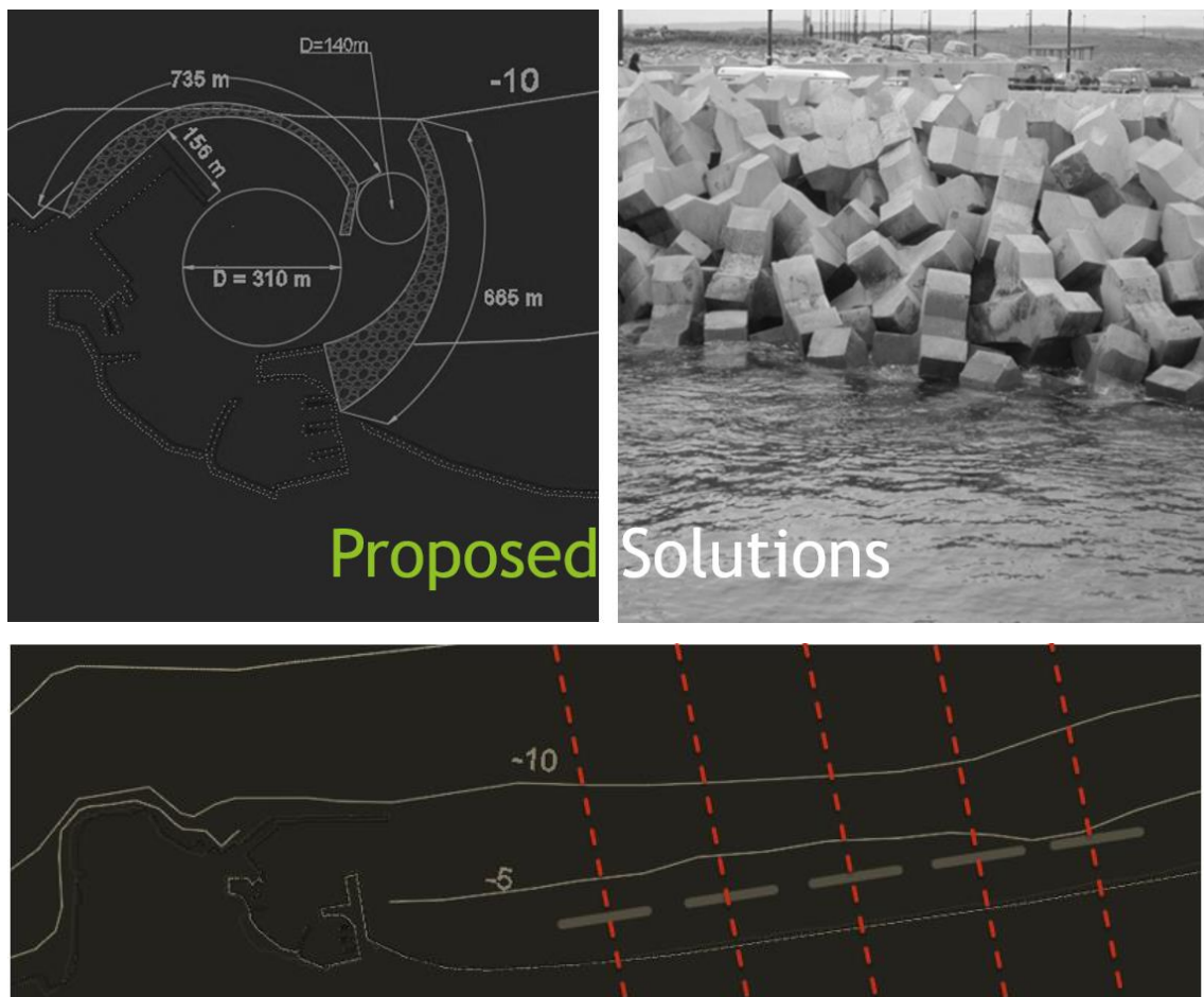
Figure 2-17 Up: reinforcement of the breakwater’s embankment and alteration of the harbour geometric properties. Down: Scheme of the projected system of submerged detached breakwaters along the coast.
