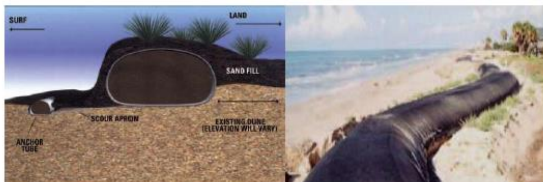
Figure 1-7 Section of a geotextile tube which placed along the beach to reinforce the sand dune (Source: Geotubes®)
