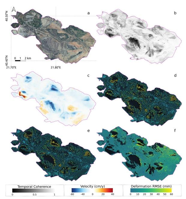
Figure 2.10 Cross-comparison of the deformation results in the mining region (denoted with purple polygon). a) Google earth optical image at 2018 b) Temporal coherence from Mintpy c) Average velocity (deformation rate) from Mintpy d) Stamps-Giant deformation RMSE map e) Stamps-Mintpy deformation RMSE map f) Mintpy-Giant deformation RMSE map.
