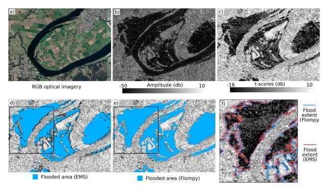
Figure 4.7 Geometric distortions of EMS product (EMSR504) a) Optical Google earth imagery. b) Amplitude which is the product of backscatter coefficients of VV and VH in decibel at flood date. c) T-scores of the Sentinel-1 intensity dataset. d) EMS results overlaid over the t-score image. e) FLOMPY results overlaid over the t-score image. f) Flood extents between FLOMPY and EMS products.
