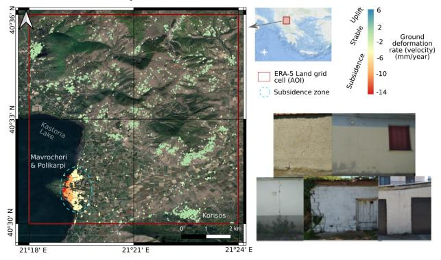
Figure 2.12 Area of interest (left), ground deformation rate information (left) and in-situ photographs of buildings located inside subsidence zone (bottom right).
