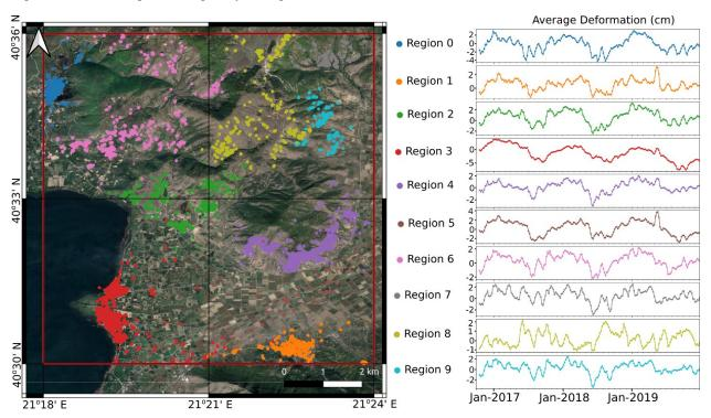
Figure 2.15 Clustered ground deformation results (left), Average deformation over time for each cluster/region
