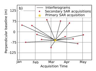
Figure 2.1 Interferogram network types a) fully connected network for Mintpy, Giant and Stamps/MTI approaches b) single master network for Stamps-PS approach
