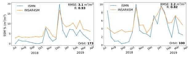
Figure 3.4 InSAR4SM SSM (volumetric %) estimations vs FordDryLake ISMN SSM (volumetric %) observations
