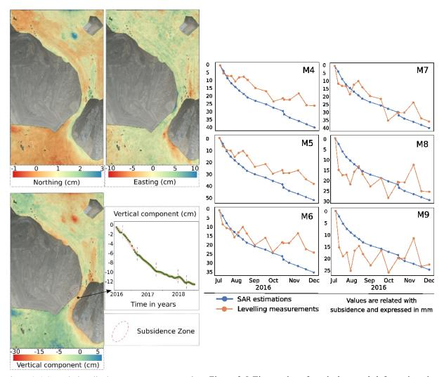
Figure 2.4 Cumulative displacement components from Figure 2.5 Time series of vertical ground deformations in 10/1/2016 to 5/7/2018. Time series of displacement correspondence of six locations the subsidence zone. The inside the subsidence zone (bottom right).
