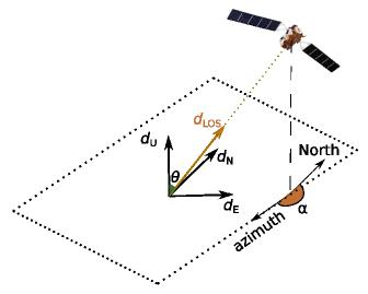
Figure 2.2 The SAR imaging geometry and the relationship between LOS deformation and the vertical, North-South and East-West components.  $\theta$  and  $\alpha$  are the radar incidence angle and the orbit azimuth angle, respectively.
