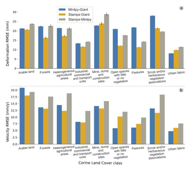
Figure 2.9 Deformation (a) and deformation rate (velocity) (b) RMSE values for each Corine land cover level-2 class in the AOI.
