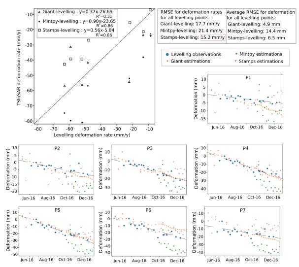
Figure 2.11 Comparison of TSInSAR accumulated displacement (subsidence) results with in-situ measurements for seven levelling points (position of the levelling point $\sigma$  given in Fig 2.6). Levelling values are projected in the LOS direction for the comparison.
