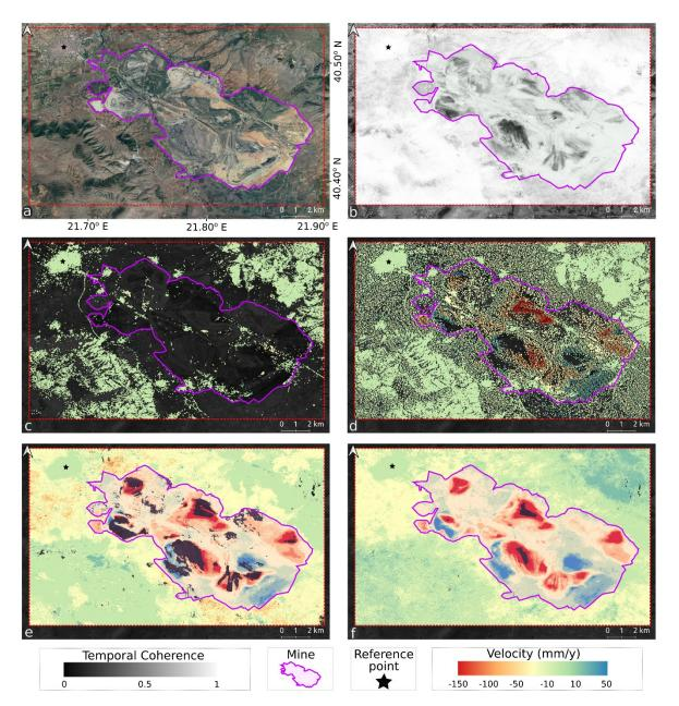
Figure 2.8 LOS deformation rate results of open source TSInSAR approaches. a) Google earth optical image at 2018. AOI is denoted with the red dashed rectangular. Mining region is denoted with purple polygon. b) Temporal coherence of the SAR dataset from Mintpy. c) Stamps Permanent Scatterers (PS) results d) Stamps/MTI results e) Mintpy-WSBAS results f) Giant-NSBAS results. Red color indicates subsidence while blue showing uplift.
