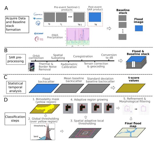
Figure 4.2 Flowchart of the four-step proposed methodological pipeline (FLOMPY).
