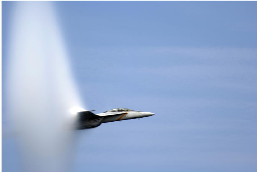
Figure 1.5: An F/A-18E Super Hornet reaches the speed of sound As the airplane reaches the speed of sound, a sonic wave is formed. In the image it is the white mist that surrounds the aft part of the plane. (photo courtesy of Jesse L. Dick [11])
