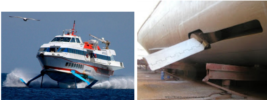
(a) A Hydrofoil vessel during planing operation [7]
