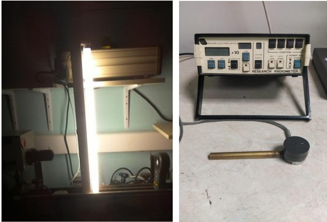
Image 7. Establishment of indoor lighting characterization setup: A luxmeter (left) and a radiometer (right) were used at set distances away from the fluorescent lamp, in order to create an equivalence relationship between lux (luxmeter) and irradiance (radiometer)
