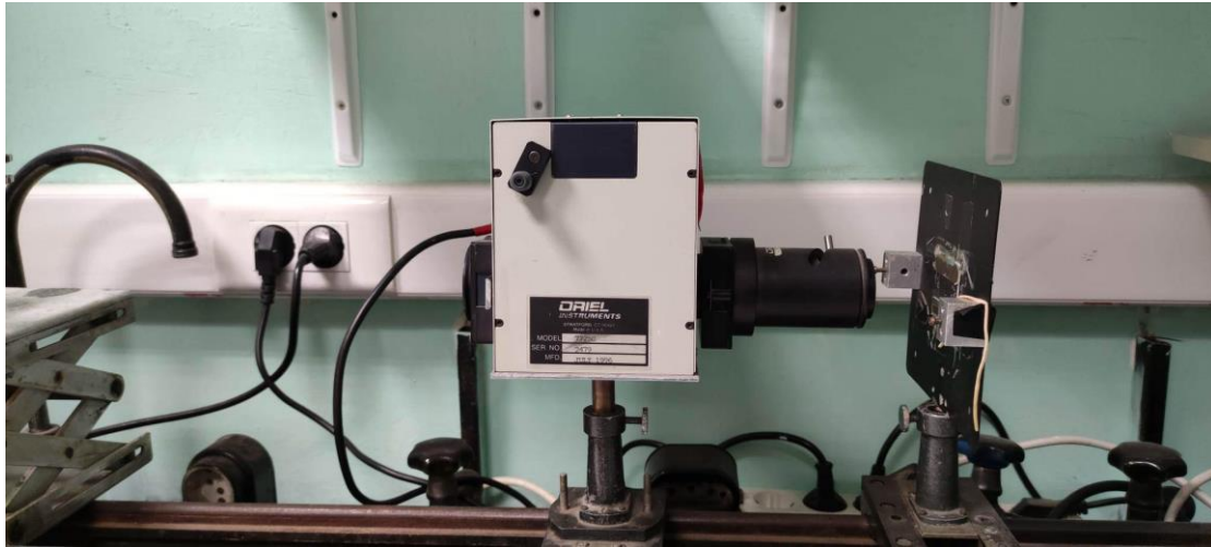
Image 4. Monochromator setup used for the IPCE characterization of the solar cells.
