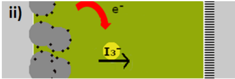
Fig. 3 i) Cycle of regeneration in a I/I_3^- electrolyte-based DSSC ii) Recombination of TiO_2 CB electrons to triiodide ions.
