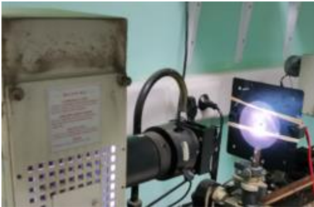
Image 5. Xenon lamp with (top) and without (bottom) neutral density filter, for the simulation of 1 sun ( 100 \text{ mW/cm}_2 ) and 0.1 sun ( 10 \text{ mW/cm}_2 ) of light intensity, respectively
