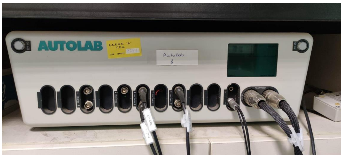
Image 3. The Autolab PG-STAT-30 potentiostat used for the characterizations of the solar cells.
