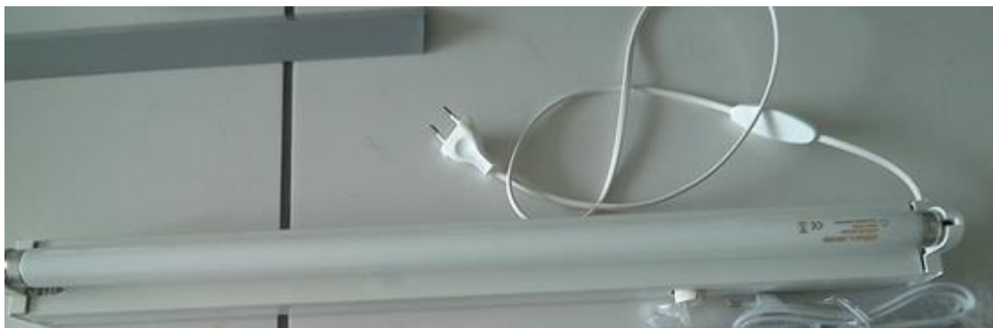
Image 6. The fluorescent lamp used for the simulation of indoor lighting environments.
