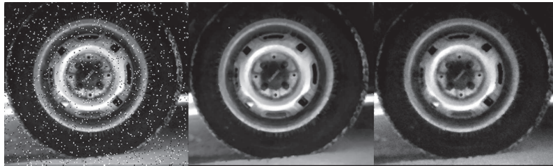
Figure 6.7: Denoising using a 3 \times 3 median filter. From left to right: I) MATLAB's 8-bit noisy image with salt & pepper noise density 0.05, II) MATLAB's median filtered image, III) Proposed stochastic median filter with sequence length N = 256 and register size m = 3 -bits.
