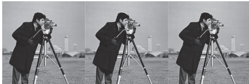
Figure 6.4: Image Sharpening Filter. From left to right: a) MATLAB's Original Image, b) MATLAB's Image Sharpening calculation, c) Image Sharpening Filter realized with the proposed SC architectures. Sequence length N = 256 and register size m = 4 -bit.
