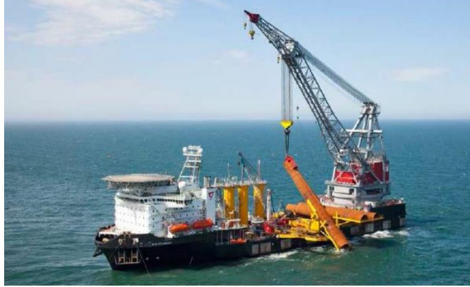
Figure 8: Cargo transportation of monopiles [5].
