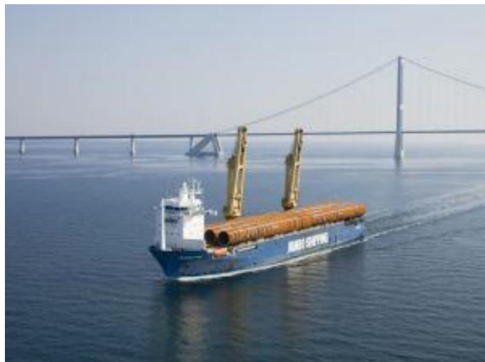
Figure 9: Monopile transportation on an offshore supply vessel [5].
