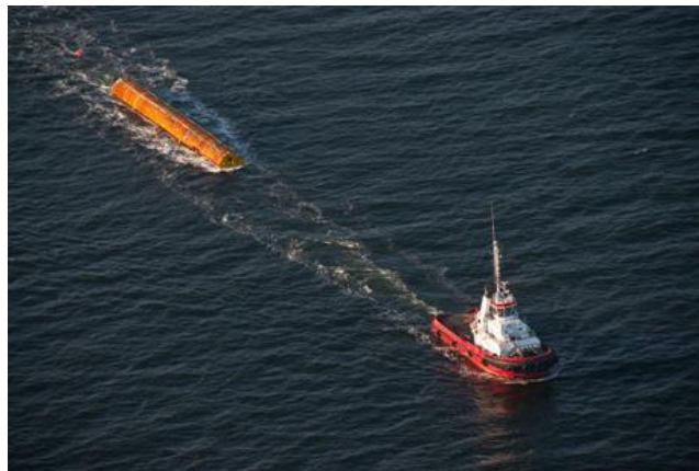
Figure 7: Monopile floating transportation [5].
