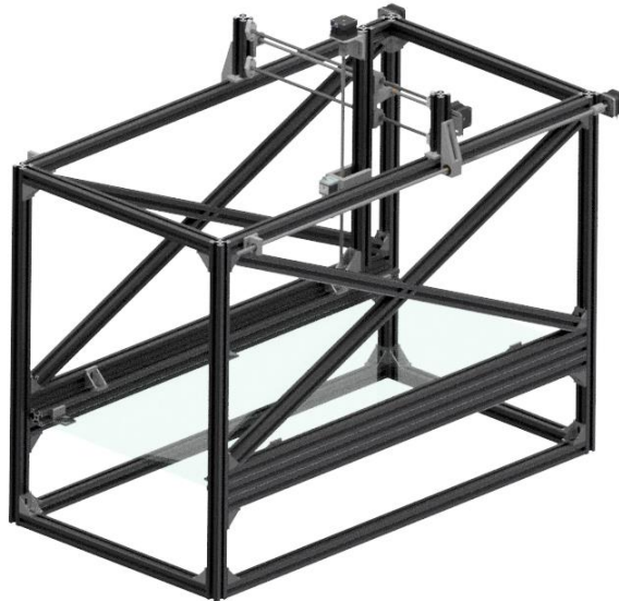
Figure 48: Proposed design with diagonal aluminum extrusions
