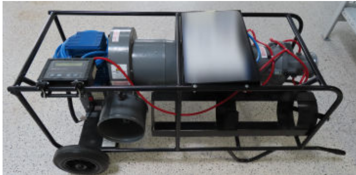
(a) Airflow Generator
