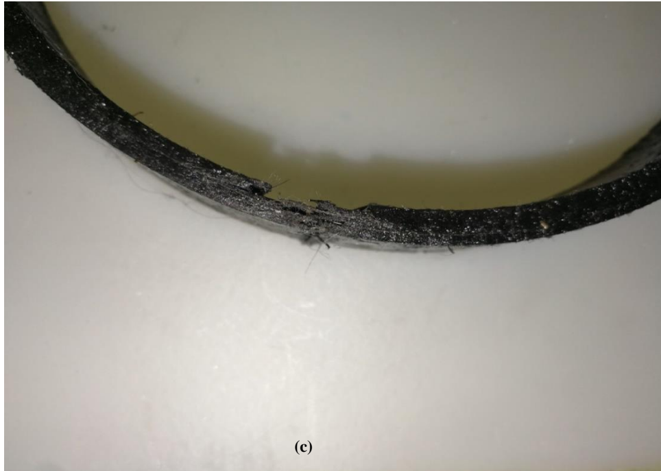
Figure 3.14 (a) outer surface of broken specimen where \pm 80^\circ plies are visible (b) inner surface of specimen where fractured \pm 12^\circ plies are also visible (c) signs of delamination in the middle plane through thickness of the specimen
