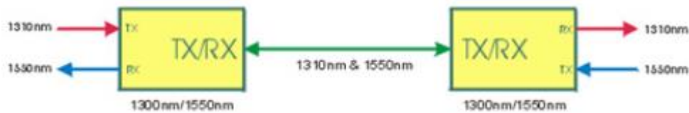
Figure 2.46 Schematic representation of bidirectional signal multiplexing configuration using two separate wavelengths
