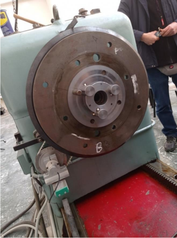
Figure 4.4 (a) Movable end plateau with the adapter mounted (b) Angle measurement system (digital clinometer)
