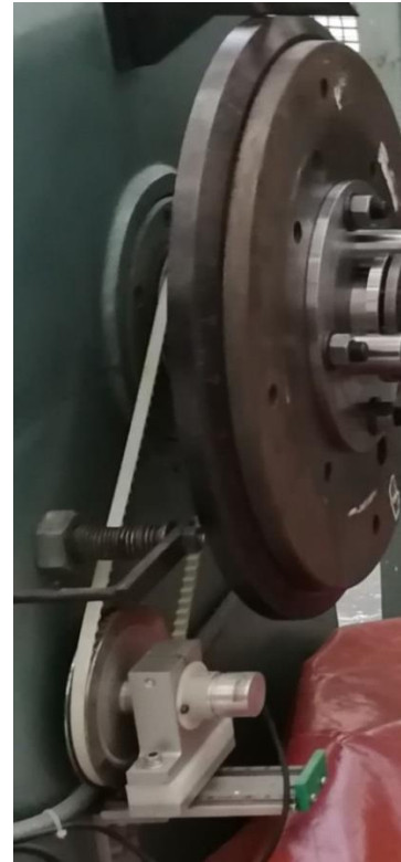
Figure 4.4 (a) Movable end plateau with the adapter mounted (b) Angle measurement system (digital clinometer)
