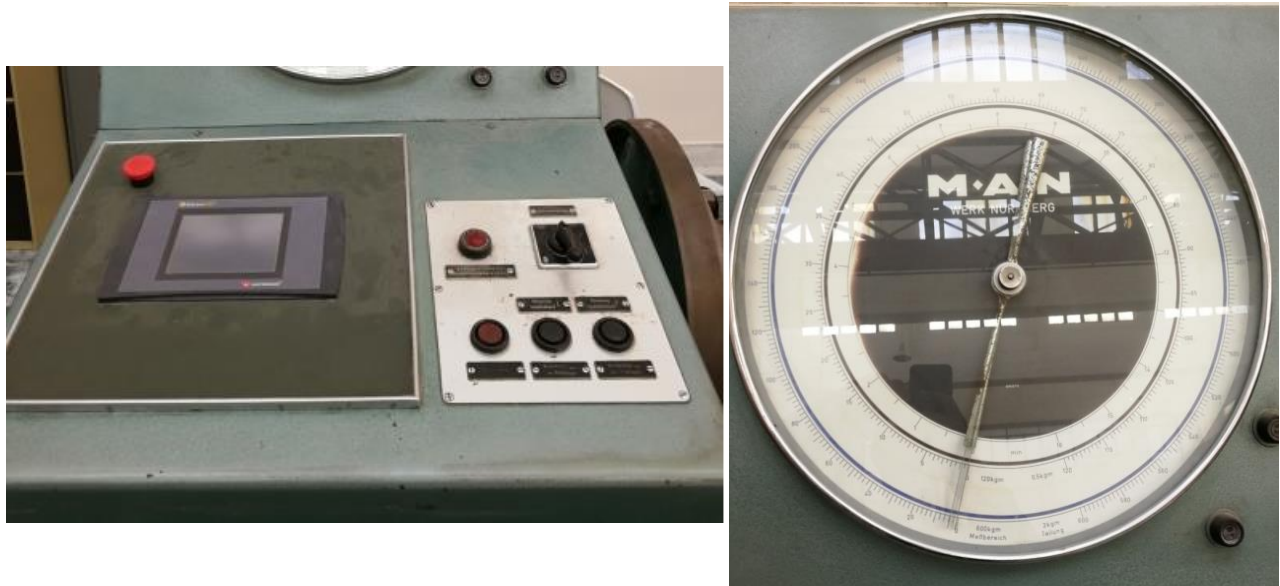
Figure 4.6(a) Control panel of machine (Vavatsikos) (b) Analog torque measuring system (Vavatsikos)
