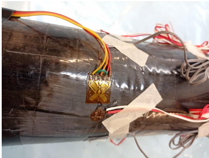
Figure 4.8 L/2 longitudinal position of shaft where the following sensors are visible: single, four-element shear strain (TorqueTrak 10K) and biaxial strain gauges
