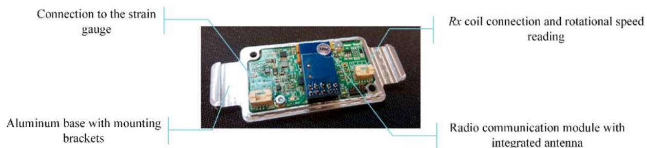
Figure 2.69 Non-stationary part and its components (Bonislawski et al. 2019)
