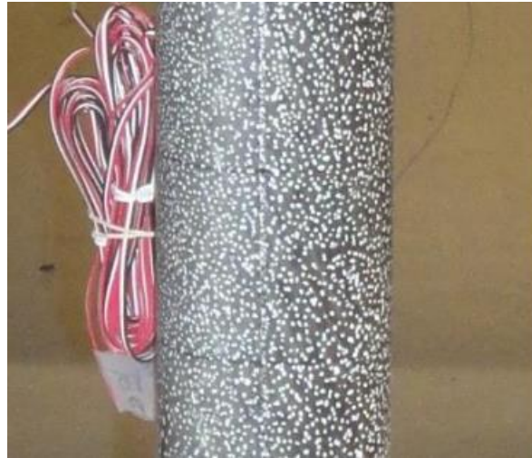
Figure 2.64 Random speckle pattern on a composite tube in Shadmehri & Hoa (2019)
