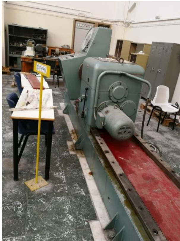
Figure 4.3 Torsional test machine of the LTM (Vavatsikos 2020)
