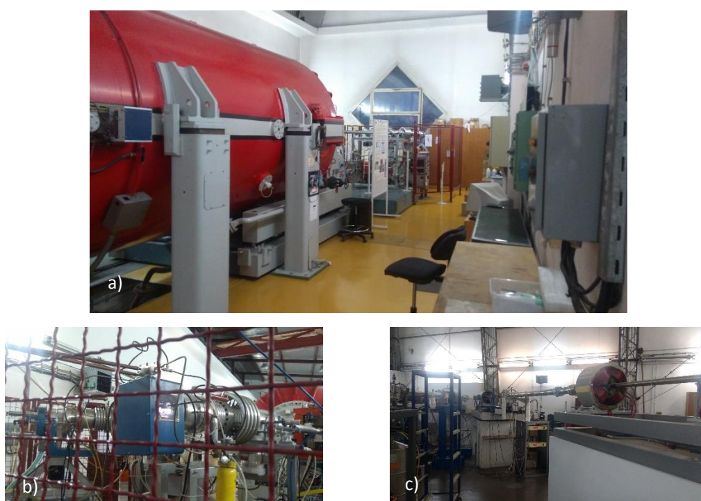
Figure 25: a) The Van der Graaff accelerator, b) the source of the ^3\text{He} and c) the experimental line for the micro beam measurements at Ruđer Bošković Institute, in Zagreb.
