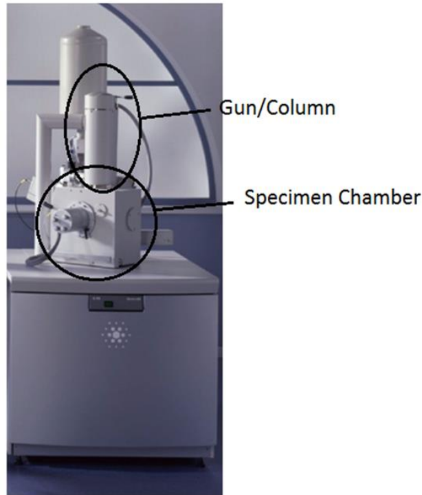
Figure 38: The experimental setup of the SEM technique.
