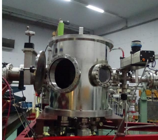
Figure 23: The chamber for the ion milli-beam measurements of Tandem Accelerator at NCSR “Demokritos” in Athens.
