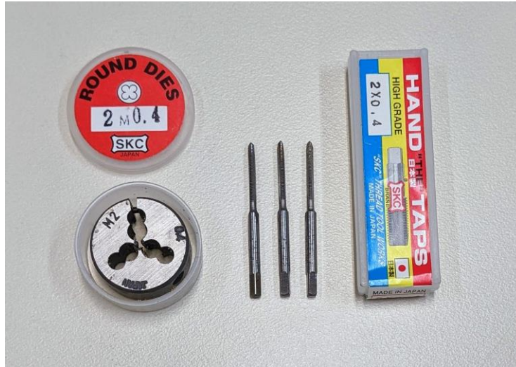
Figure 3-19. Tap and Die used by the watchmaker for the manufacturing of the lead screw system.
