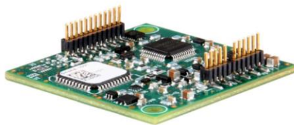
Figure 3-38. Motor Driver for the slave motor (for the complete Datasheet see Appendix A).
