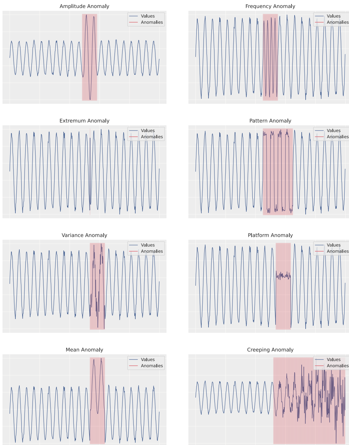
Figure 3.7: Examples of each anomaly type taken into consideration for the development of the synthetically generated time-series datasets.
