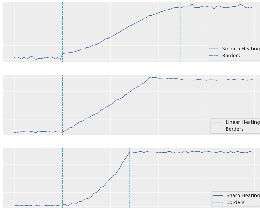
Figure 5.15: Three different segments portraying the depicting a scrubber tower's heating process over different time windows, with different behaviours.
