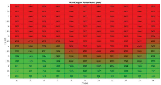
Figure 2. WaveDragon power matrix (kW).
