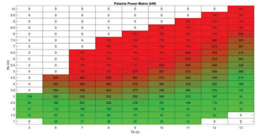
Figure 1. Pelamis power matrix (kW).
