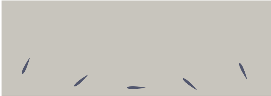
Figure 1.6 Motion Example of a fully passive energy harvesting flapping foil.
