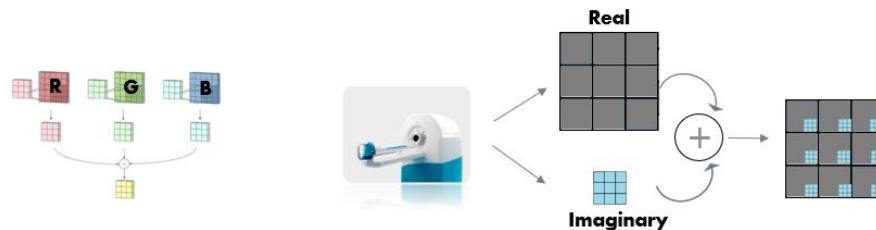
Fig.3.7: A. CNN operation on 3 Channel colour input (RGB). B. Complex MRI analogy – The two parts are intentionally presented with such a big size difference to denote the order of magnitude difference in real sampled data.
