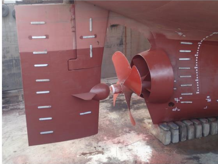
Figure 62: Mewis Duct installed in Vessel 2
