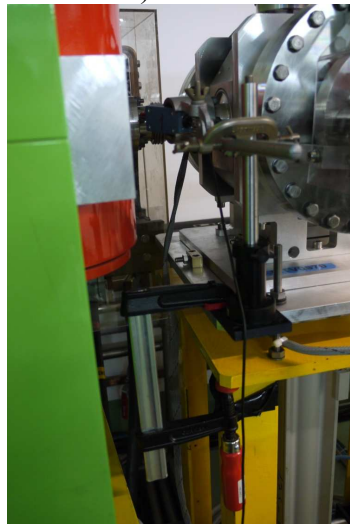
Figure 70: The OTR screen upstream side
