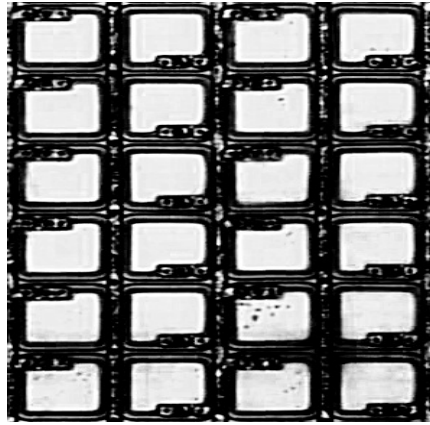
Figure 59: Black and white zoom in the SiPM in order to have a preliminary estimation of the fill factor.
