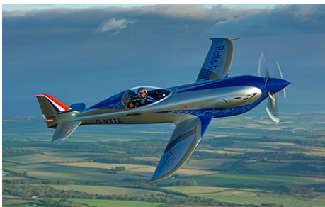
Σχ. 1 “Spirit of Innovation”, Rolls-Royce, 3x Axial flux motor (3x 790Nm, 200kW), speed_{max} > 550\text{km/h}
