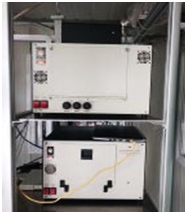
Figure 14: Semi-continuous organic and elemental carbon aerosol analyzer, “Demokritos” Laboratory.
