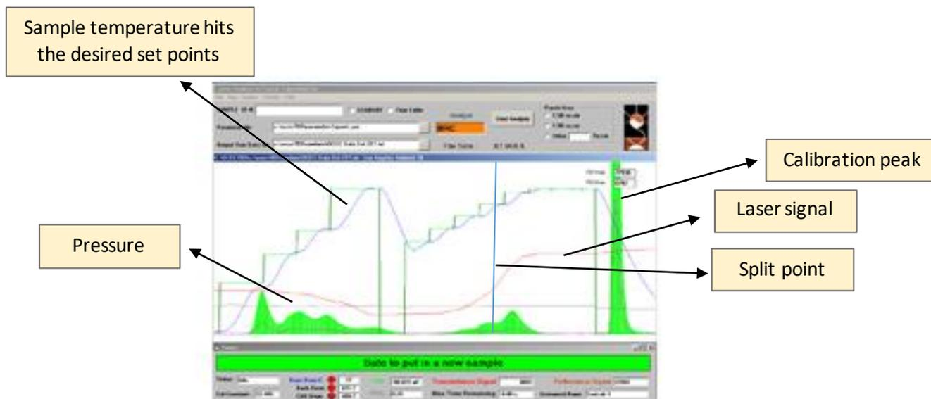
Figure 12: Thermograph of OC/EC analysis for EUSAAR2.
