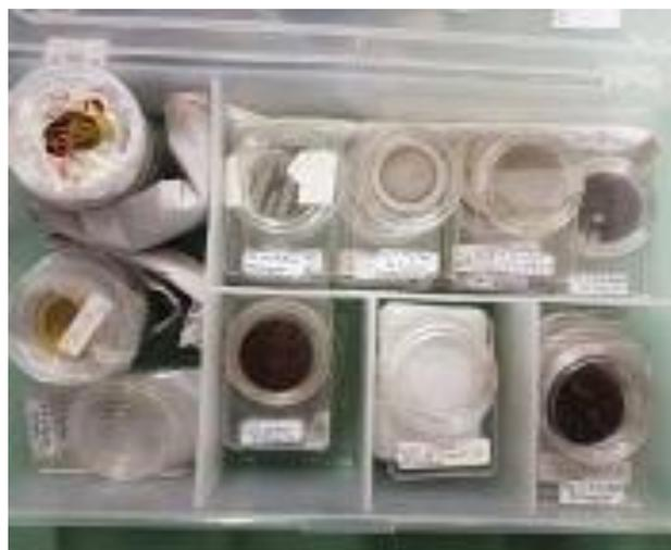
*Figure 18: Prototype filters for ED-XRF Epsilon 5 PANalytical calibration.*
