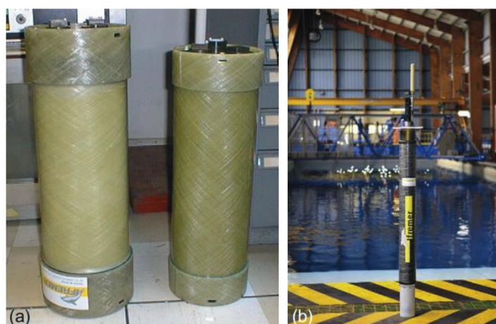
Figure 1.4 Oceanographic instrument protection casings (a) Glass/epoxy filament wound housings (500mm long, 150mm inner diameter) (b) Deep Arvor profiler engaged in ARGO project (1000mm long, 100mm inner diameter) (Davies, 2016)
