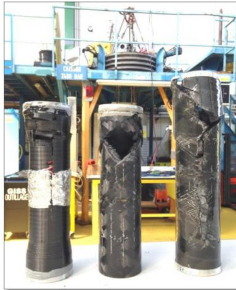
Figure 1.33 Composite cylinders after implosion tests. From left to right (i) C/PA6 [\pm 0^\circ/88^\circ] , (ii) C/PA6 [0^\circ/\pm 55^\circ] , (iii) C/Epoxy [\pm 55^\circ] (Arhant et al., 2009)
