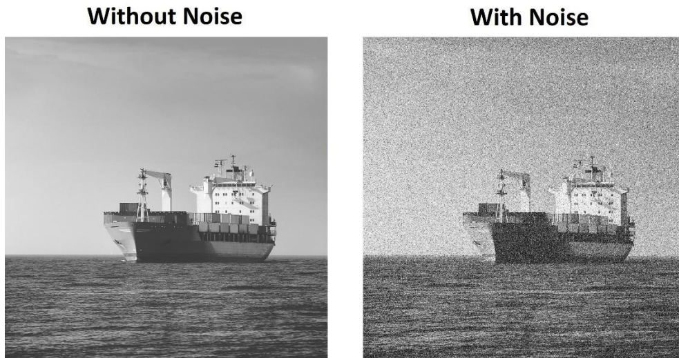
Figure 3.8 Noise Generation using the Gaussian Model for \sigma=0.5
