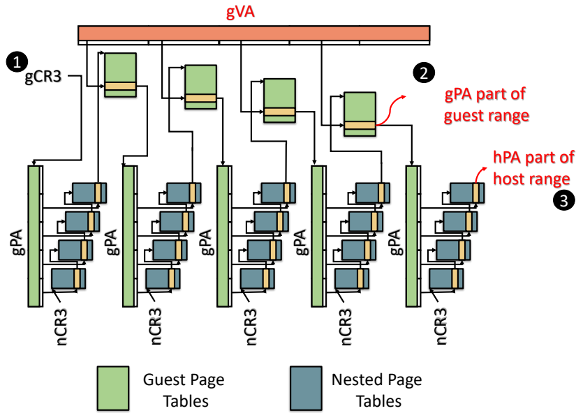
Figure 4.10: Range TLB miss in vRMM. Part1: The nested page walker identifies the missing page translation and if the page is part of a guest and host range.
