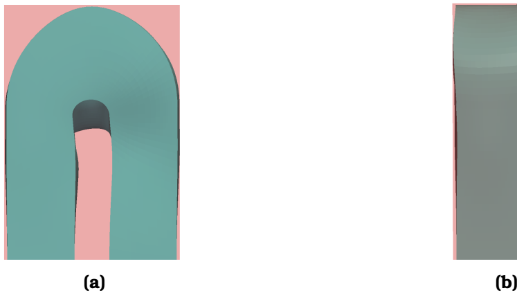
Figure 5.15: U-Bend Duct: Two perspective views of the final shape resulting from the constrained optimization. The duct is in blue while the bounding box in transparent red.
