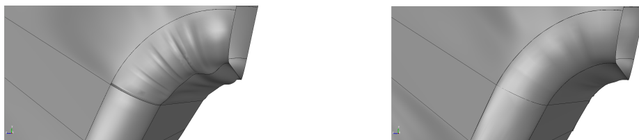
Figure 5.33: Comparison of the optimal shape resulting from the constrained (right) and the unconstrained (left) optimization of the S-bend duct.
