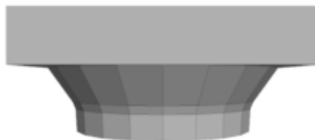
Figure 73: Simulation of the column capital as a single block, without damages, in 3DEC
