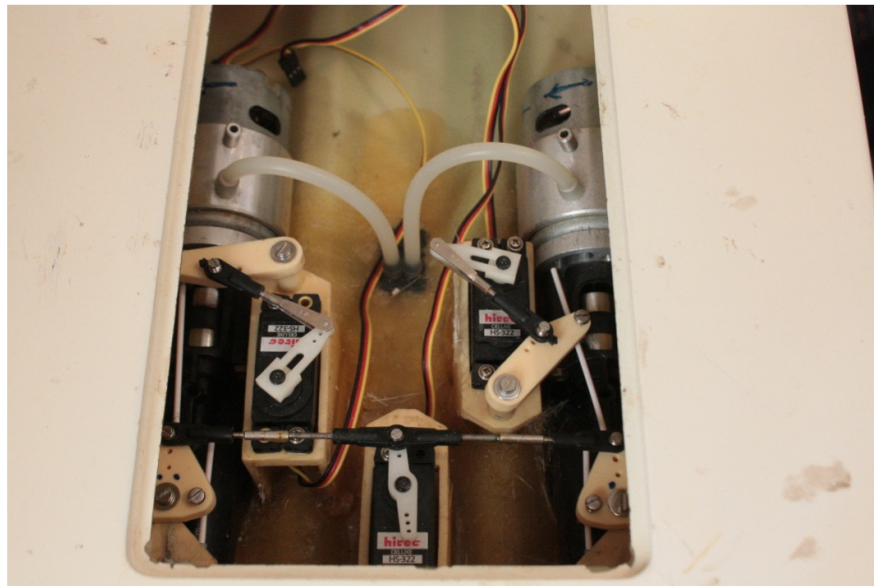
Figure 3: Waterjet servo-controls and propulsion motors.
