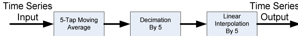
Figure 13: Signal processing to generate smooth yaw acceleration signal for the neural nets in the continuous-time state model.
