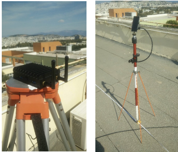
Figure 6.16: Wi-Fi RTT access point (left) and Android device (right) outdoors setup for the static 1D ranging part of Campaign C#0.3
