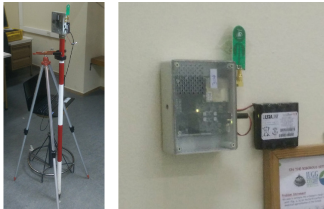
Figure 6.19: Time Domain® UWB modules during C#1 field testing - mobile node located at point C3 (left) and anchor node attached on the wall (right)
