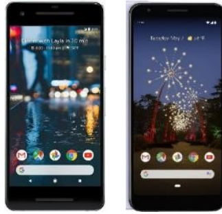
Figure 6.3: Wi-Fi RTT enabled Android smartphone devices. Google Pixel 2 TM (left) and Google Pixel 3a XL TM (right)
