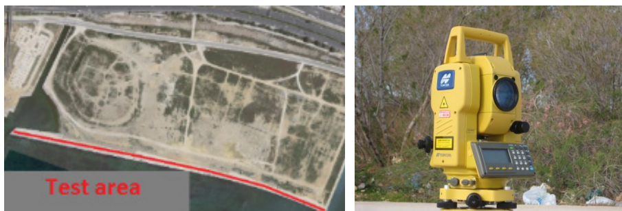
Figure 6.13: Faliro test area top-view (left), total station Topcon GPT 3107N (right) of Campaign C#0.1
