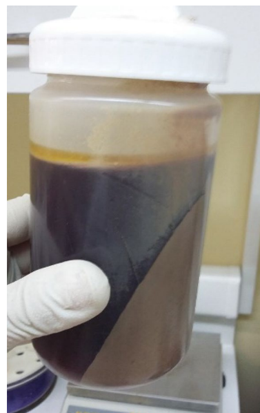
Fig. 1 Generation of the three phases after the acidification/hydrolysis and the centrifugation process (upper phase: residual oil; middle phase: aqueous phase rich in phenolic compounds and sugars; bottom phase: remaining solids)
