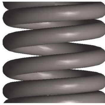
Figure 6.14: Five coil helical spring used to realize the negative stiffness element
