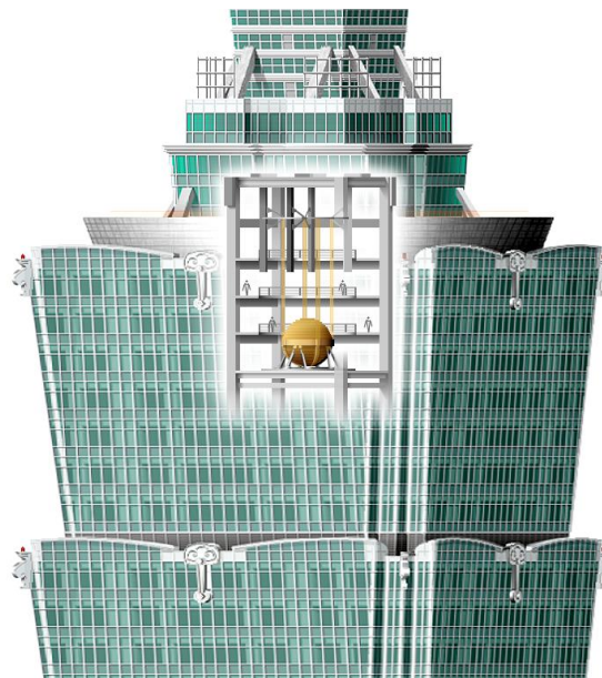
Figure 2.3: Tuned Mass Damper (TMD), installed on top of the Taipei 101 Tower in Taiwan
