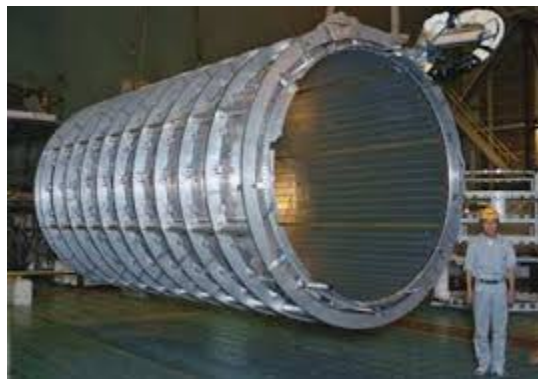
Figure 2.7: The Central Solenoid magnet
