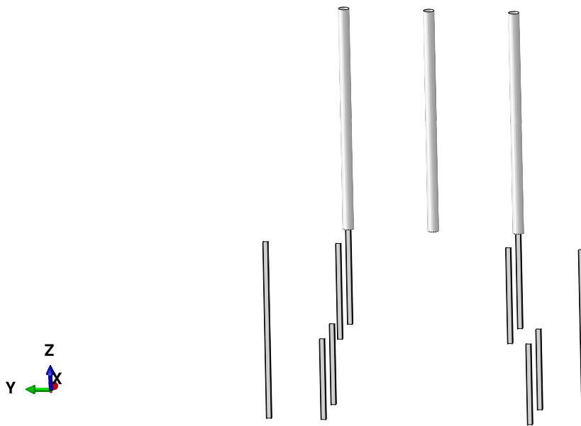
Figure A.9: Aft view of vertical stiffeners in Abaqus/CAE environment
