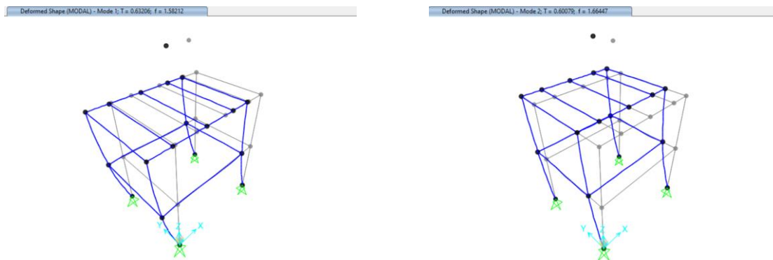
Figure 3.88 Modal analysis of the roof water tank – (a) T_x = 0.63 sec, T_y = 0.60 sec
