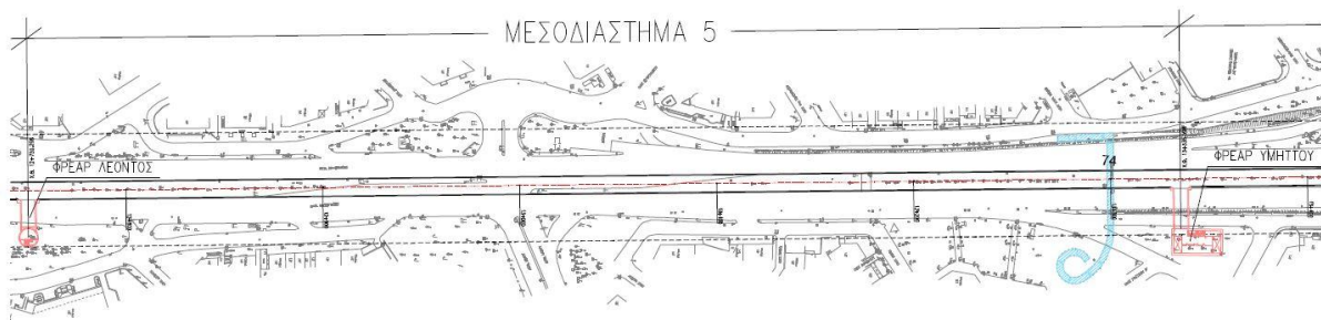
Figure 3. Plan view of the TBM tunnel from shaft “Leontos” to shaft “Hymettus” TBM interval 5. Existing constructions within the tunnel influence zone (Atiiko Metro S.A. 2005).
