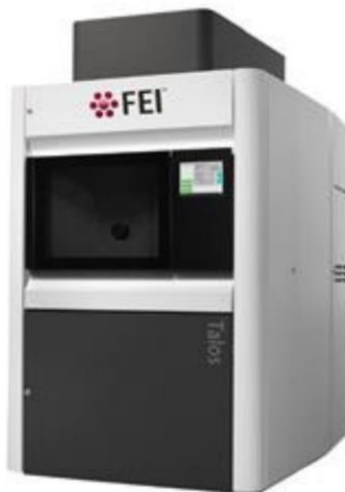
Εικόνα 5.13 Talos F200X TEM (The Pennsylvania State University, Η.Π.Α.).
