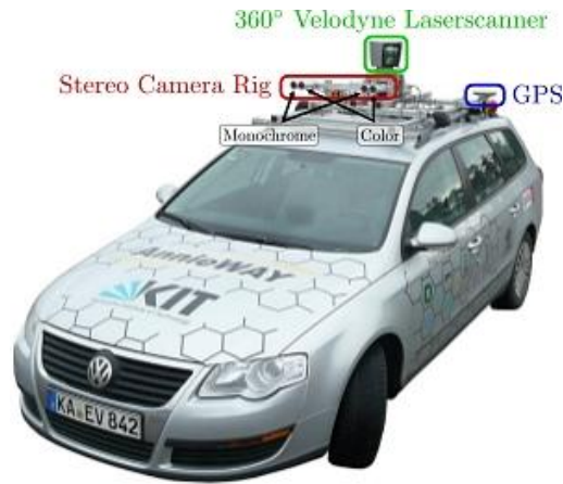
Figure 4-6. KITTI Dataset Sensors [88].
