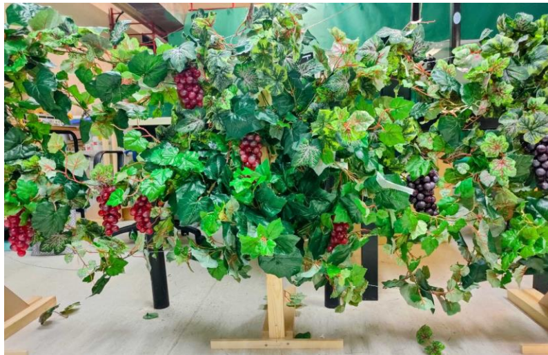
Figure 4-3. Vineyard experimental setup at CSL. The grapevine canopy consists of two leaf types with different color, i.e., green & green-yellow leaves.
