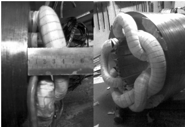
Fig. 15. Low winding head length and high filling factor
