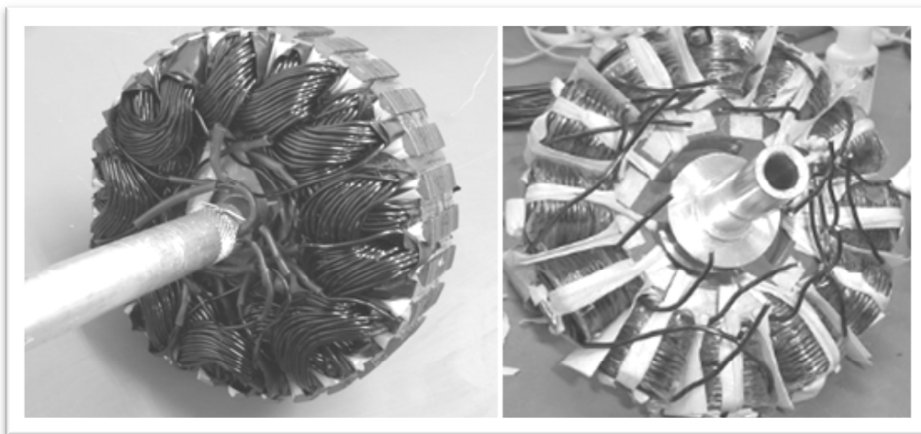
Figure 1- The two motor stators with full pitch (left) and fractional pitch (right) configurations
