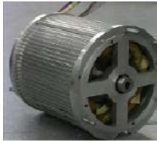
Figure 12. Assembled motor for a 60kW EV used on an existing car coach
