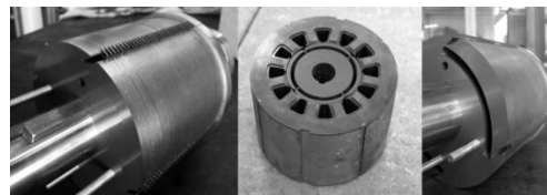
Fig. 7. The three rotor prototypes prior to mounting the PMs
