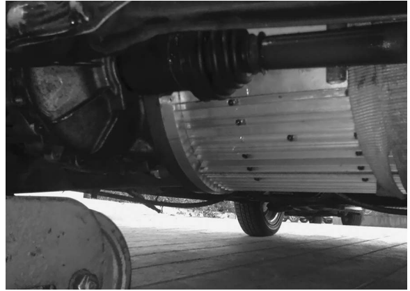
Fig. 19. Mounting process of the motor prototype to the Smart For TWO.
