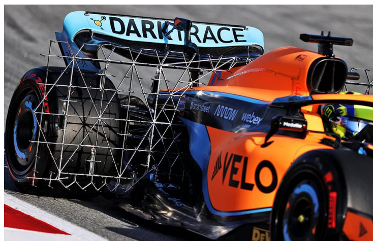
Figure 6-6 Aero Rakes, series of pitot tubes measuring pressure in F1 car ( www.wtf1.com )
