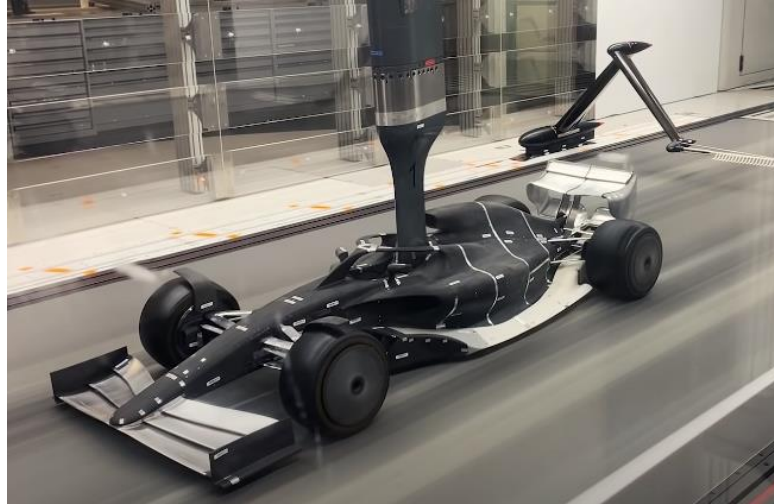
Figure 6-5: Scaled F1 Model in a Wind Tunnel ( www.formula1.com )
