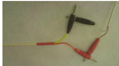
TC Long Pt18 & Type B extension wire
