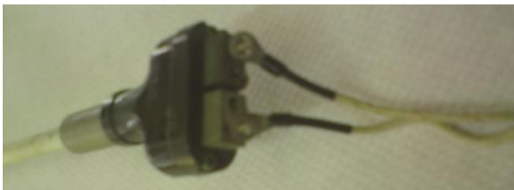
TC Type K & Blue type K extension wire
